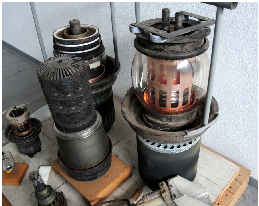
Large defective transmitting tubes -Relics from earlier times.
